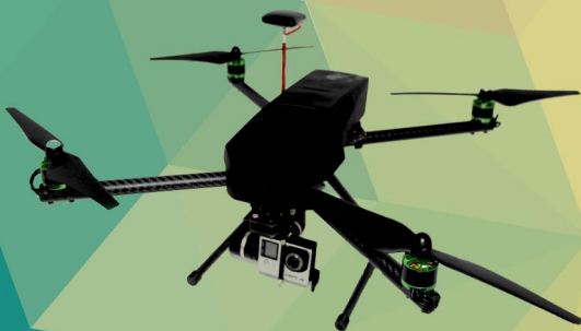
TinjauKopter Multirotor Survey Drone With Onboard Autopilot
